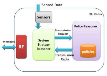
Fig. 2. XG radio architecture [1].
