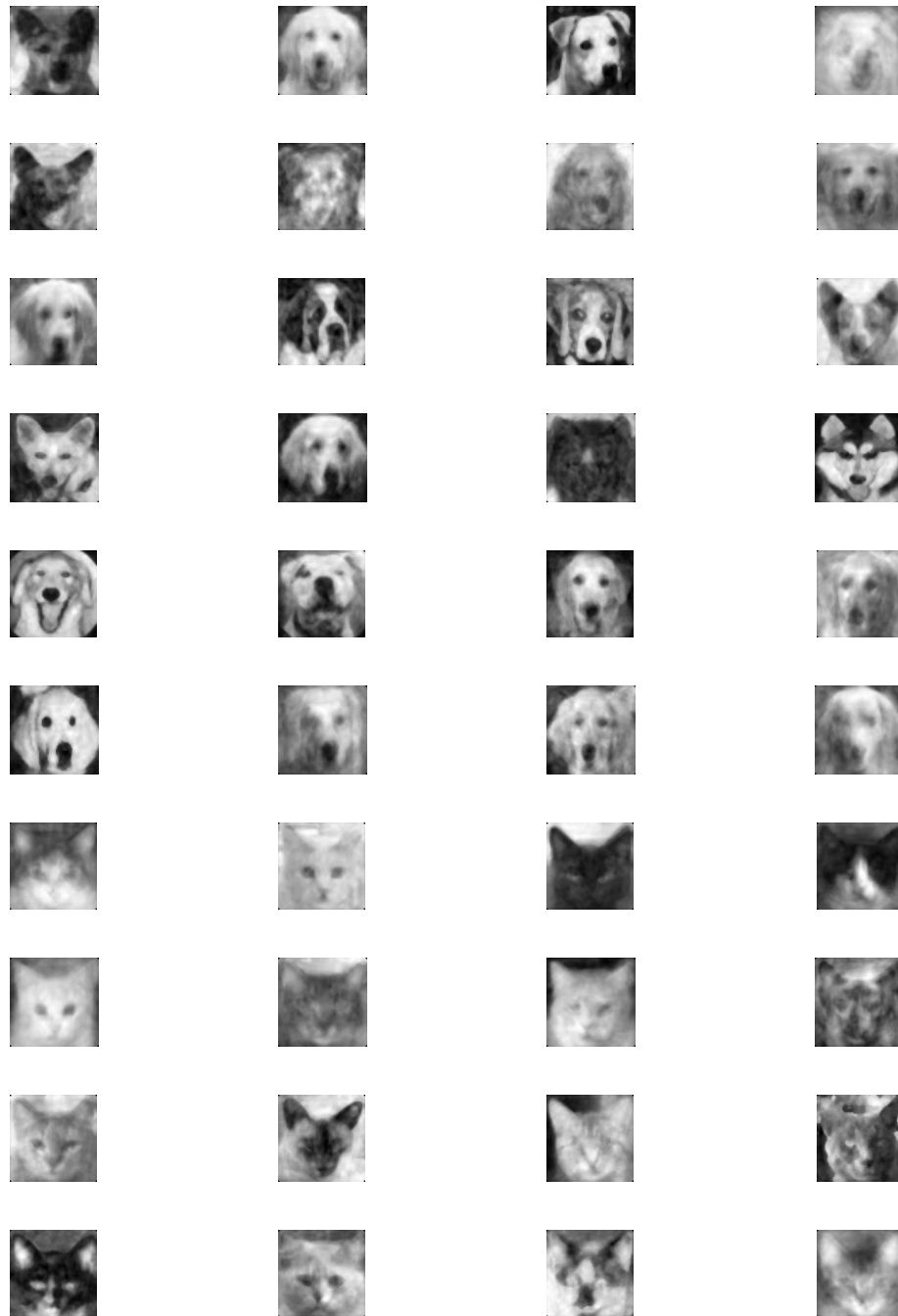
FIGURE 4.1. Self organized map on a 10 by 4 lattice for the 160 cat/dog training images. There are 24 prototype dogs, and 16 prototype cats.
