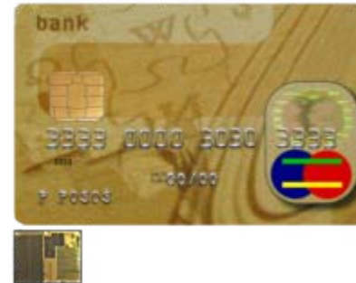
Credit card with smart-card capabilities. The 3-by-5-mm chip embedded in the card is shown, enlarged. Smart cards combine low cost and portability with the power to compute cryptographic algorithms.
