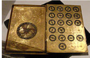
16th-century book-shaped French cipher machine, with arms of Henri II of France
