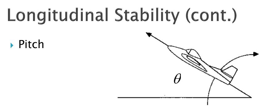
Pitch is the only parameter of longitudinal motion in an aircraft, therefore it is the only thing considered when analyzing longitudinal dynamic stability.
