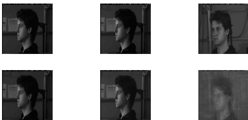
Fig. 2. Top: first principal vector for a sample probe. Bottom: first principal vector for the correct gallery set that the algorithm identifies for experiments I, II, and III from left to right. The first principal angle between the top and bottom vector is 0.066, 0.069, and 0.269 radians, from left to right.
