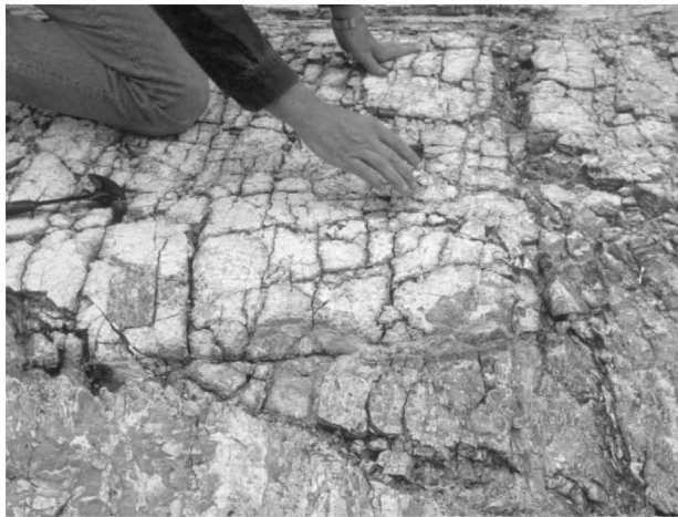
Figure LLi-03. Several distinct, but irregular joint sets in chert and porcelanite.
