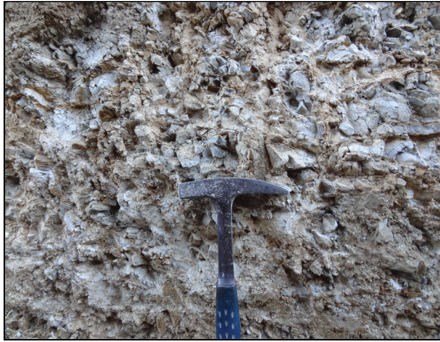
FIGURE 24. Typical calcareous silty claystone lithofacies. Note blocky to conchoidal fracture pattern without distinct bedding.
