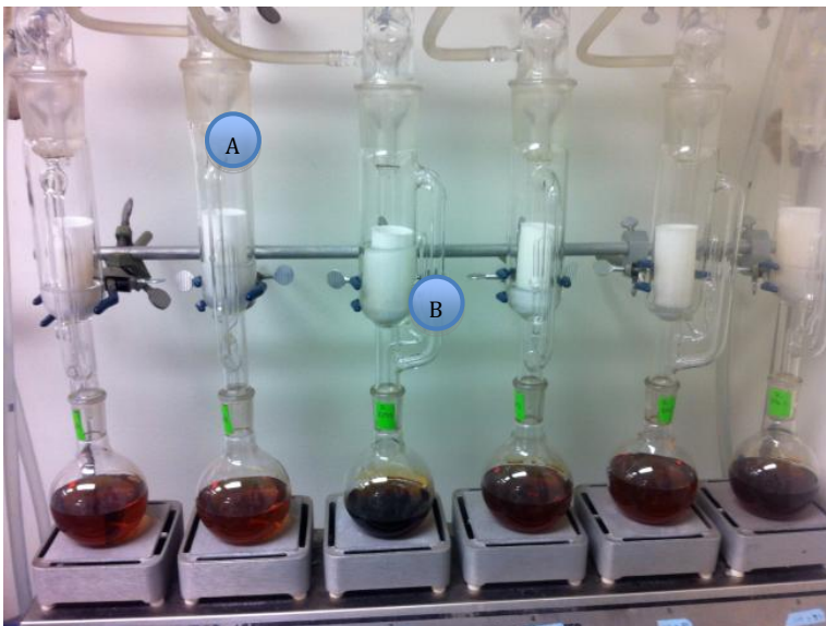
FIGURE 3.2. Soxhlet extraction for powdered core samples. A. White silicon thimbles filled with powdered core sample. B. Glass beakers filled with dichloromethane and hydrocarbons removed from each sample after extraction process is complete.
