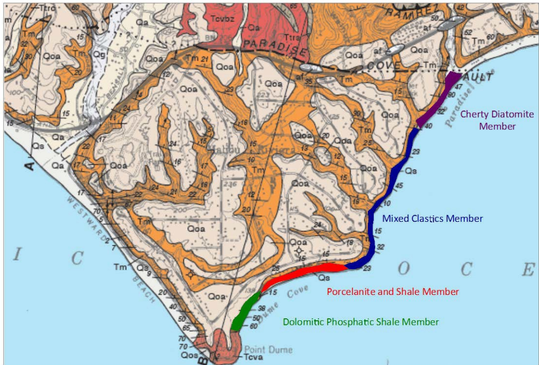
FIGURE 4.2. Extent of the four members of the stratigraphic column. Reflecting the Monterey Formation along the coastal cliffs between Point Dume and Paradise Cove. Displayed on geologic map modified from Dibblee and Ehrenspeck (1993).
