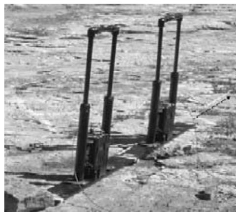
**Figure 4.** EV GPR polarization with long axis of antennae in line with survey.
