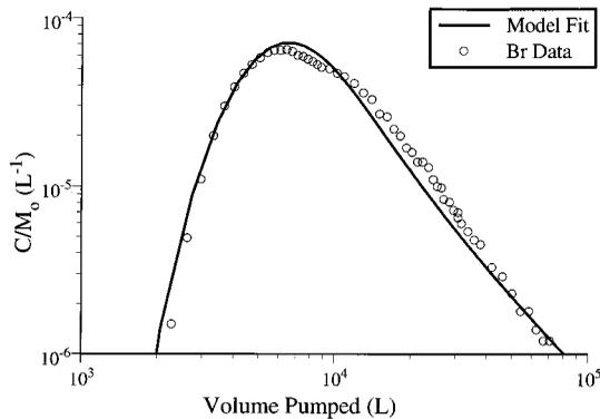
**Figure 5.** Fit of matrix diffusion model, given in the appendix, to the test C bromide breakthrough. The characteristic time of diffusion in the matrix ( $\tau_p = 1480$  min) is based on the free diffusion rate of bromide in water, and the residence time in the borehole ( $\tau_s = 546$  min) was measured. Fitted model parameters are  $Pe = 15$  and  $\tau = 1620$  min.
