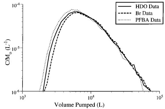
**Figure 3.** Normalized breakthrough of all tracers for test C ( $Q = 2.9 \text{ L/min}$ ).
