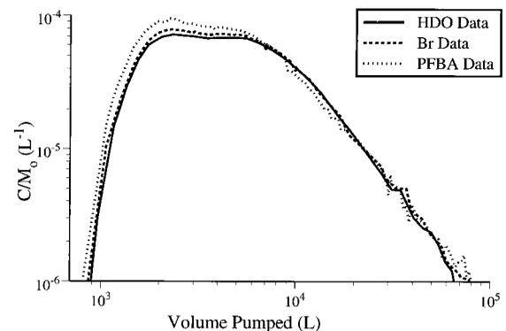
**Figure 4.** Normalized breakthrough of all tracers for test D ( $Q = 9.8 \text{ L/min}$ ).
