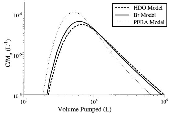
**Figure 6.** Fit of matrix diffusion model to the bromide data given in Figure 5 compared to the same model adjusted to account for molecular diffusivity of other tracers ( $\tau_p$  is 1100 and 4490 min for HDO and PFBA, respectively).
