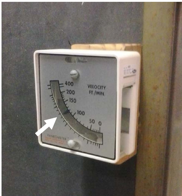
Figure 2. MICRO hood Vaneometer. Note airflow reading above 100 LFM (arrow).
