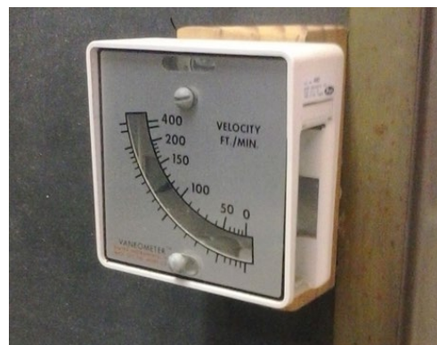
Figure 2. MICRO hood Vaneometer. Note airflow reading above 100 LFM (arrow).
