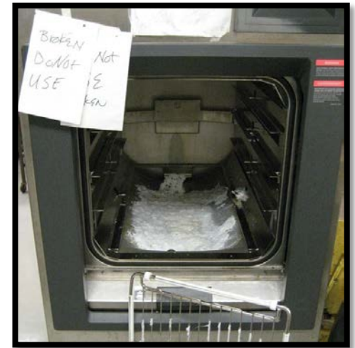
Melted Plastic: someone used non-heat stable plastic as secondary containment
