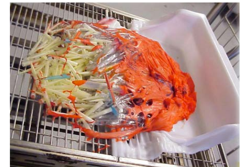
Melted Plastic: someone used non-heat stable plastic as secondary containment
